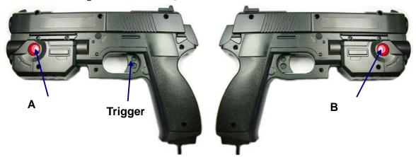
If you have bought the OEM electronics AimTrak kit then you will need to have wired up the Trigger, Aux and P1 connectors for the lightgun to work properly with Playstation 2.
